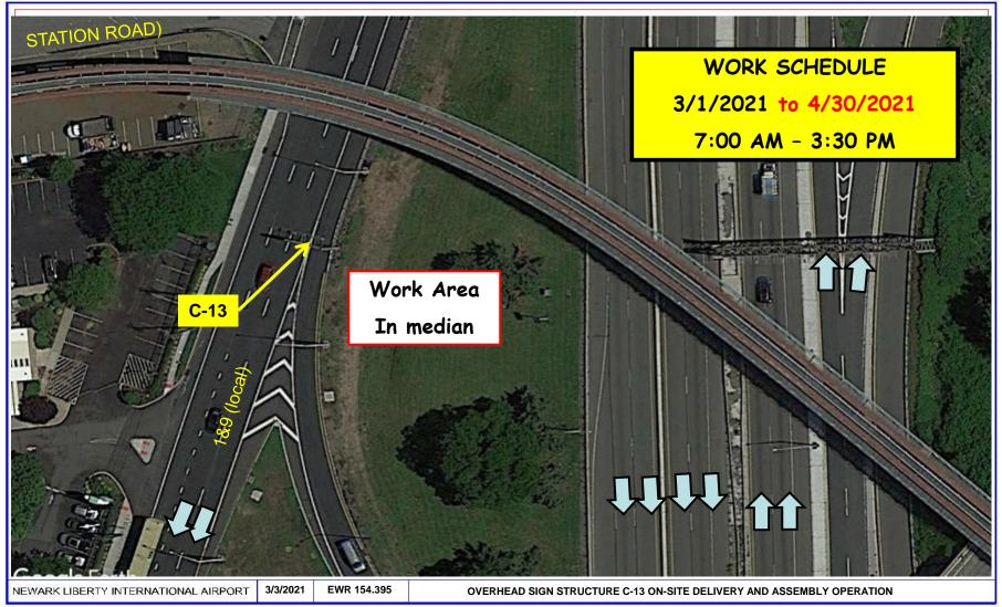
On or about Monday, March 1st, 2021 through Friday, April 30th, 2021 from 7:00 AM to 3:30 PM contractor Conti Construction/J.F. Creamer sub will perform demolition of previously installed foundation for C-13 in the grass median area behind guiderail. Equipment in use will not exceed a maximum boom height of 30 feet. All activities will be behind the guide rail in the grass median area. No lane closures will be required. Signs and PA Police will be on site.
